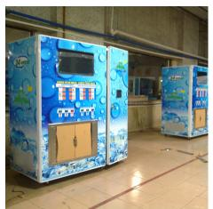
starting for using the ice. It has functions of water shortage stop protection, refrigeration system high-voltage protection, automatic selling ice and adjustable ice thickness. Commercial ice vending machinery mainly consists of powder coated steel cabinet, coin acceptor, bill validator, system board, ice making system and ice bagging system. With this automatic ice vendor, customers can buy bagged ice by coin or IC card.
